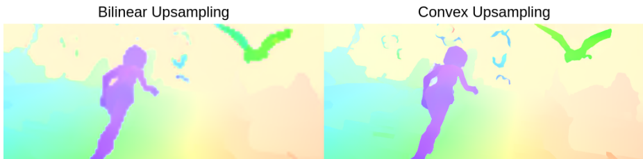
Fig. 9: Our upsampling module improves accuracy near motion boundaries, and also allows RAFT to recover the flow of small fast moving objects such as the birds shown in the figure.
